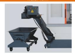
NV900 uses chip removal machine to remove debris. realizes the convenience and cleanliness of debris cleaning, improves the efficiency of waste disposal, increases the capacity of waste accumulation, liberates labor force, and provides the basis and guarantee for intelligent production. The box filter makes the water tank have a further reflux path under the same volume, and enhances the filtering effect of the water tank.
