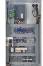
Closed electric cabinet prevents any oil and water mist from entering the cabinet, so as to avoid short circuit or damage of electrical components due to numidity.
