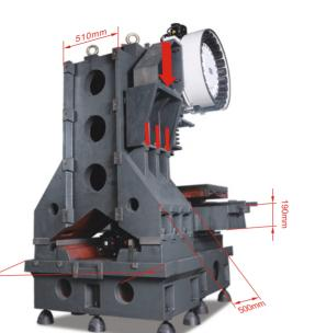
NV900 is validated by repeated analysis to ensure structural rigidity at the design stage. Compared with the traditional method, the NV900 tool base is directly loaded on the base from the column, which is not easy to deform and greatly improves the rigidity of the machine tool.
